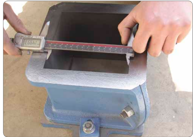
Verification of dimension using digital vernier caliper
