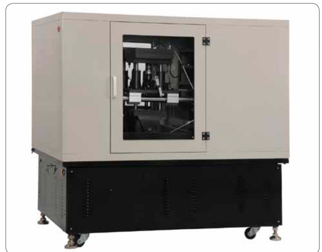
TPCT-5A wheel tracking machine
